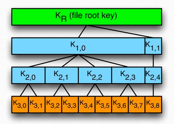
for x = start + 1 to end do  $k \leftarrow keyed_hash(k, x \parallel \lfloor b/B_x \rfloor)$ end for return k
