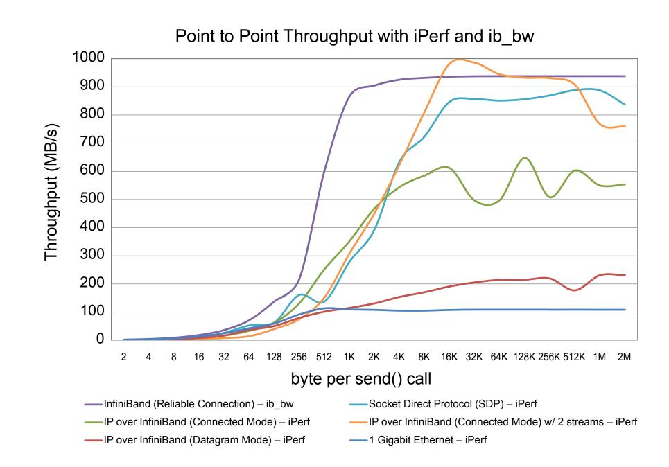
• For point-to-point throughput, IP over InfiniBand (Connected Mode) is comparable to a native InfiniBand
