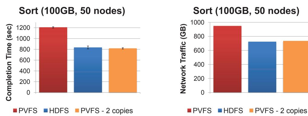
• *sort* using HDFS is faster than running *sort* on PVFS because HDFS writes the first copy locally
