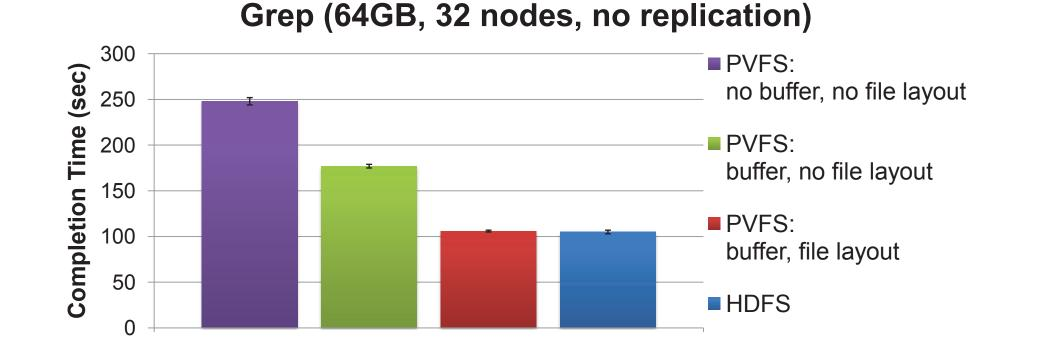
By using both readahead buffer and file layout information, PVFS performance is comparable to HDFS
