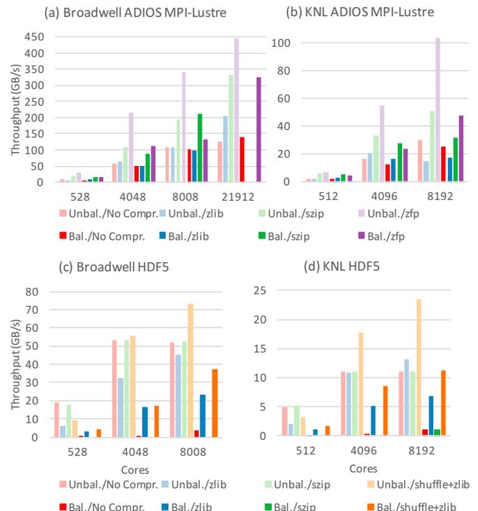
**Figure 1. A sampling of compression-assisted throughput results with two output methods on two processor types.**
